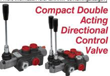
New CHIEF directional control valve for operating double acting cylinders. Ideal for small tractors and other compact applications. Features include monoblock construction, built-in adjustable pressure relief valve, load check, spring centering spool action, open center, side inlet/outlet ports, top work ports and vertical or horizontal handle mounting.
