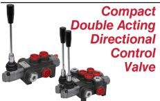
New CHIEF directional control valve for operating double acting cylinders. Ideal for small tractors and other compact applications. Features include monoblock construction, built-in adjustable pressure relief valve, load check, spring centering spool action, open center, side inlet/outlet ports, top work ports and vertical or horizontal handle mounting.
