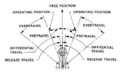
Characteristics: OF - Operating Force; PT - Pretravel; OT - Over Travel; DT - Differential Travel; RF - Release Force; OP Operating Position; TF - Travel Force; RP - Release Position; TT - Total Travel
