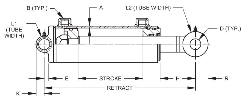
Rods are sized for a maximum safe push load (2:1 safety factor) given in the table. This is based on the pin configuration shown with no center support.
