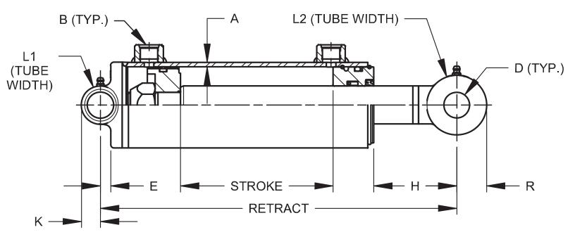
Rods are sized for a maximum safe push load (2:1 safety factor) given in the table. This is based on the pin configuration shown with no center support.
