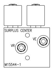
Connect VE to the extend port of the remote outlets on your tractor or to the work ports of a double acting valve, whichever applies.
