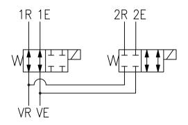
**Open Center and Closed Center Circuits**: Valve can be used as a selector valve to make a single set of outlets act like two. Use a SPST switch to power both solenoids at the same time.
