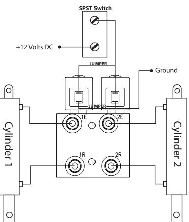
A SPST (Single Pole Single Throw) switch can be used to switch the solenoids. Power both solenoids at the same time.
