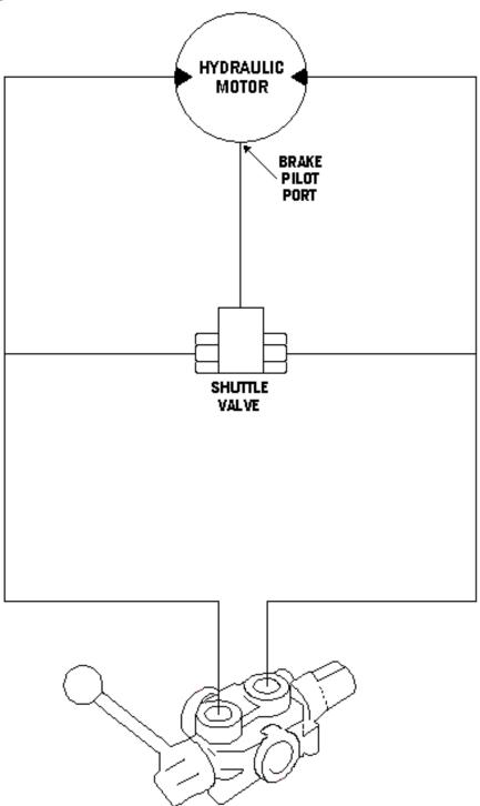
Hydraulic ball-type shuttle valves are for use as a load-shuttling directional selector. The floating ball checks to the low pressure side. Commonly used to direct oil from the high pressure side of a bi-directional hydraulic motor to a pressure-released hydraulic brake.
