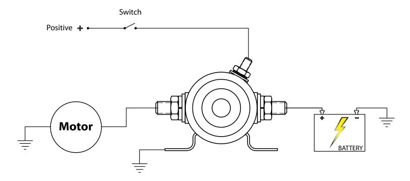
Note: Be sure to remove any paint between the solenoid and the piece you are mounting it to. Without a good ground this unit will not function properly.
