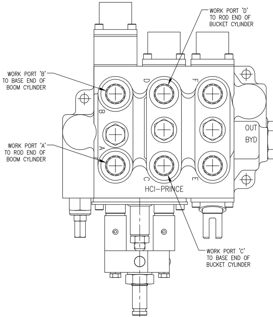
INSTALL VALVE WITH PORTS ON TOP
