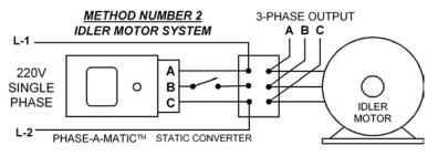
**NOTE: Mount converter upright** with the junction box on the top. The sideway diagram as shown here is to suit the illustration space only.
